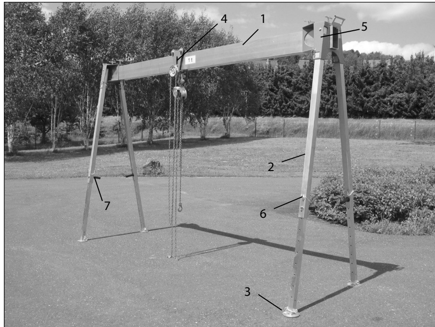
Aluminium crane with trolley and hoist unit
